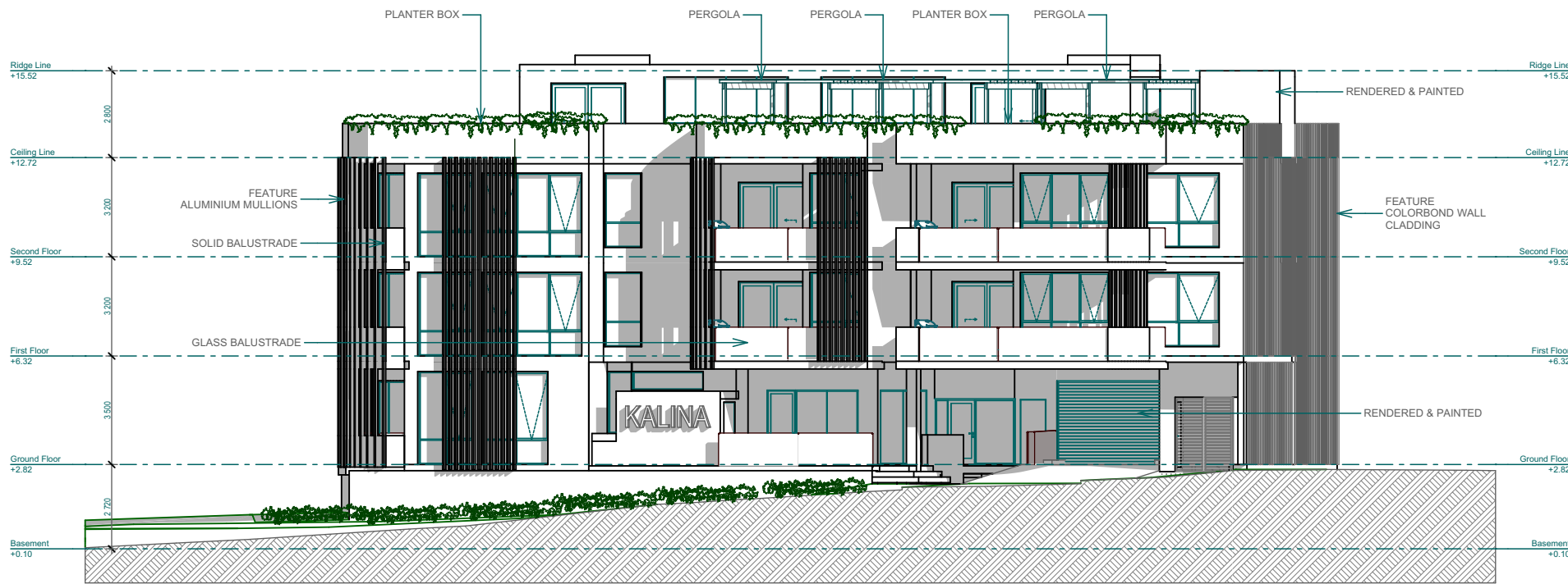
South West Elevation 1:200
